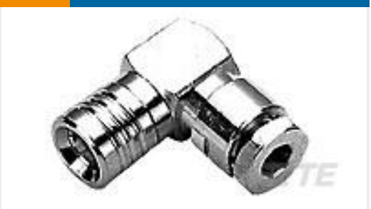
TE Part #1-1478008-0 SMB R/A Plg PS 50Ohm Gold Pltd RG174A/U,
