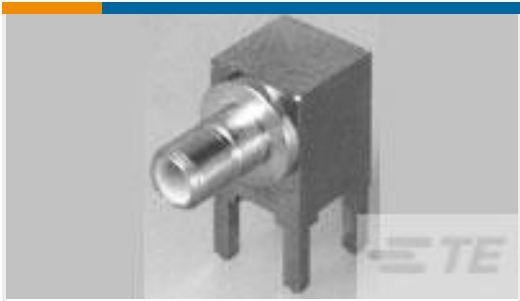
TE Part #5414337-1 JACK,RTANG,SMB/PCB
