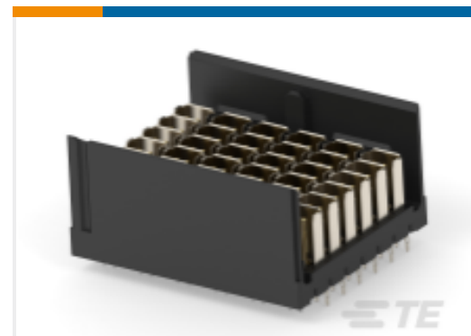
TE Part # 2187809-1 SW PIR HDR BP, 92OHM, 6X6 OE GR
